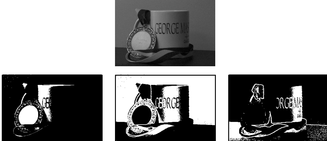
Figure 1a. An original input image. Figures 1b-d are three pulse images from the UCM.
